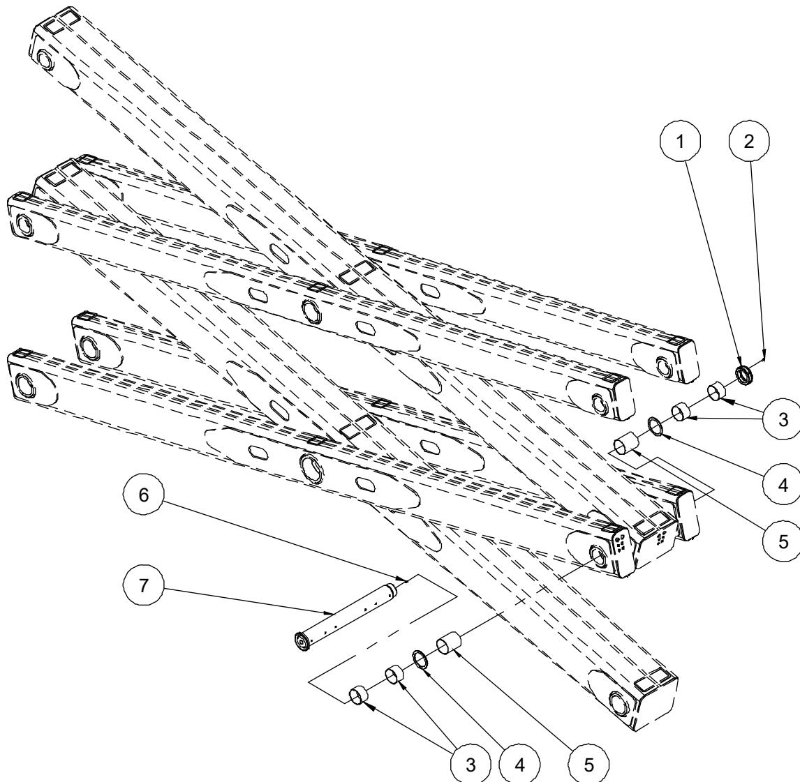
**714.1 Automatic Lubrication Systems - Scissor Arm pin joint H**
