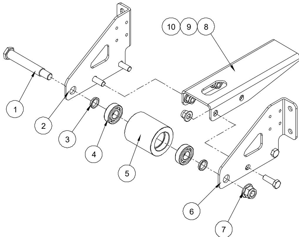
**303.2 Support Roller Assembly (Extended Platform)**
