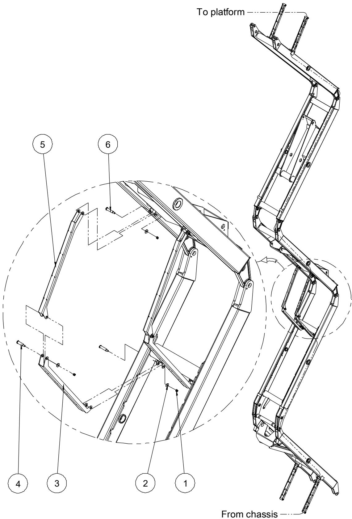
**207.1 Cable Routing Device Assembly**
