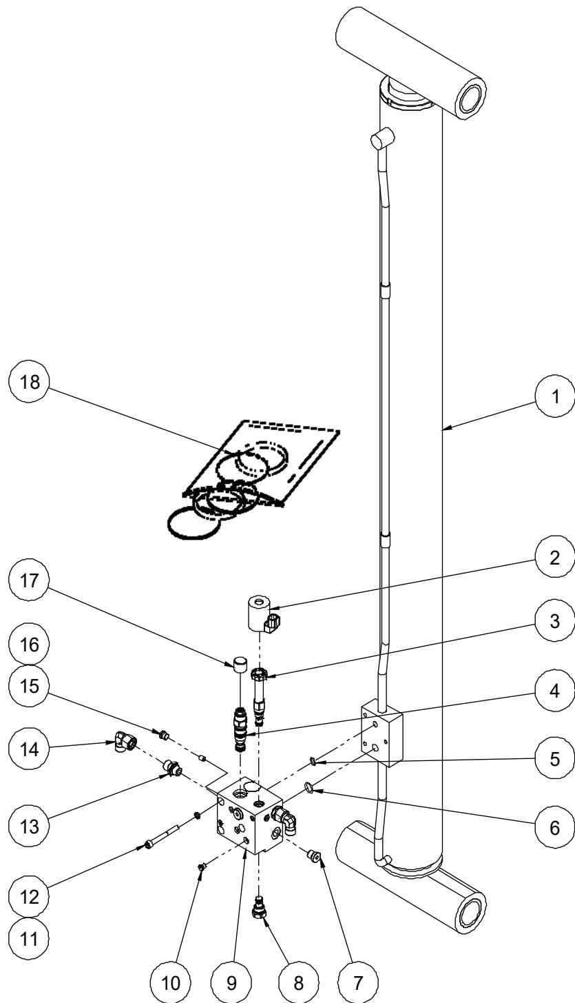
**402.1 Upper Lift Cylinder Assembly (JCPT1823RTL)**
