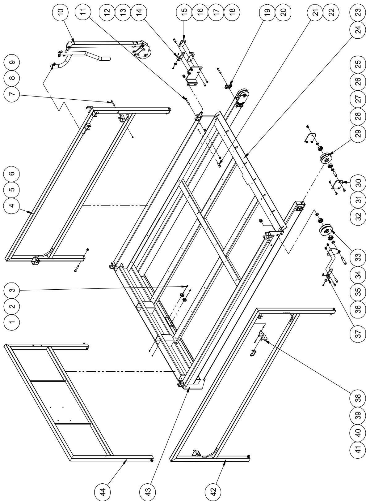
**305.1 Front Platform Extension Assembly (Standard Platform)**
