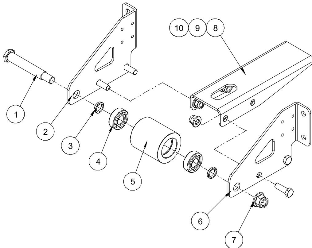
**303.2 Support Roller Assembly (Extended Platform)**
