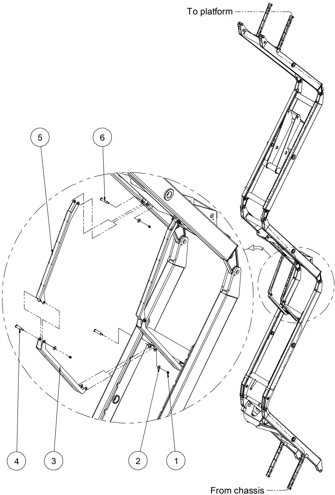
**207.1 Cable Routing Device Assembly**
