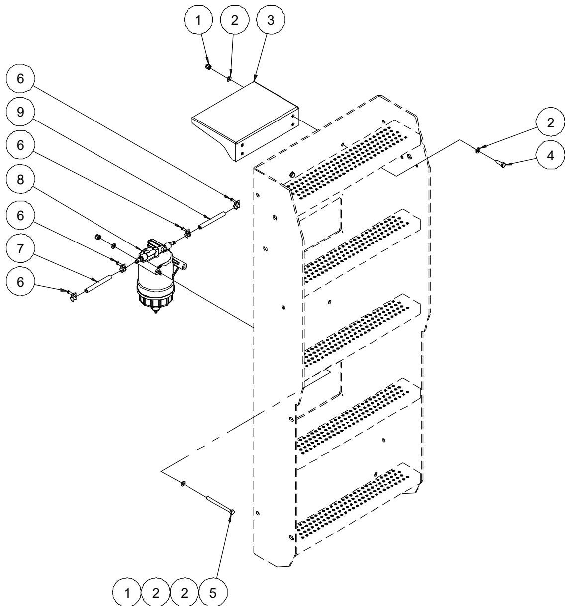
**115.3 Fuel Filter Assembly (YANMAR EU Stage V Engine)**
