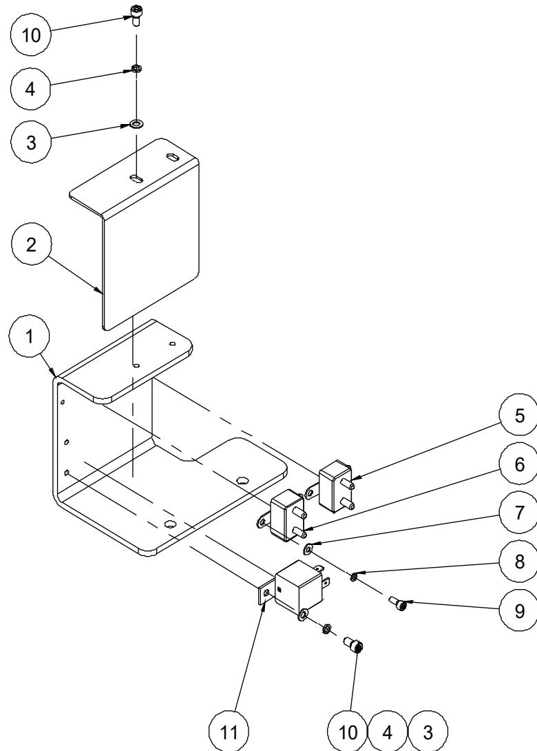
**110.3 Electrical Accessory Assembly (YANMAR EU Stage V Engine)**
