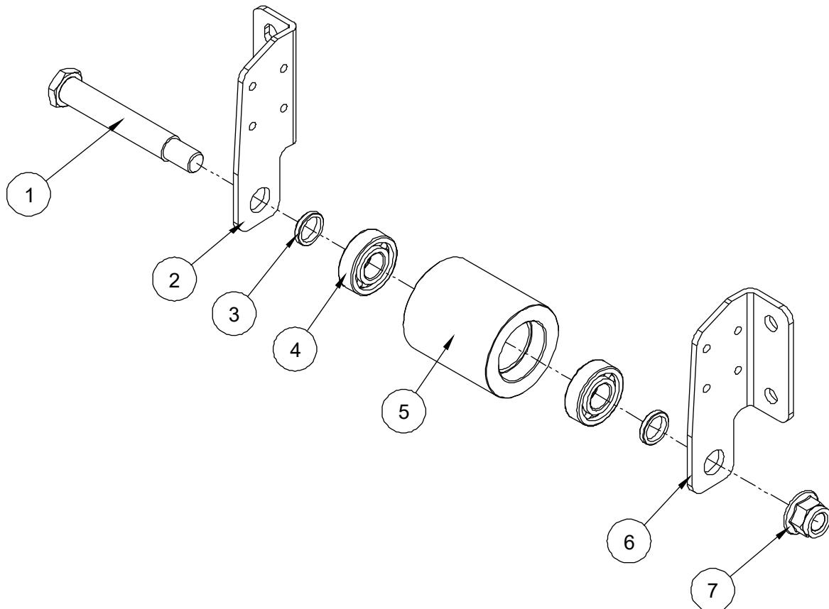
**303.1 Support Roller Assembly (Standard Platform)**
