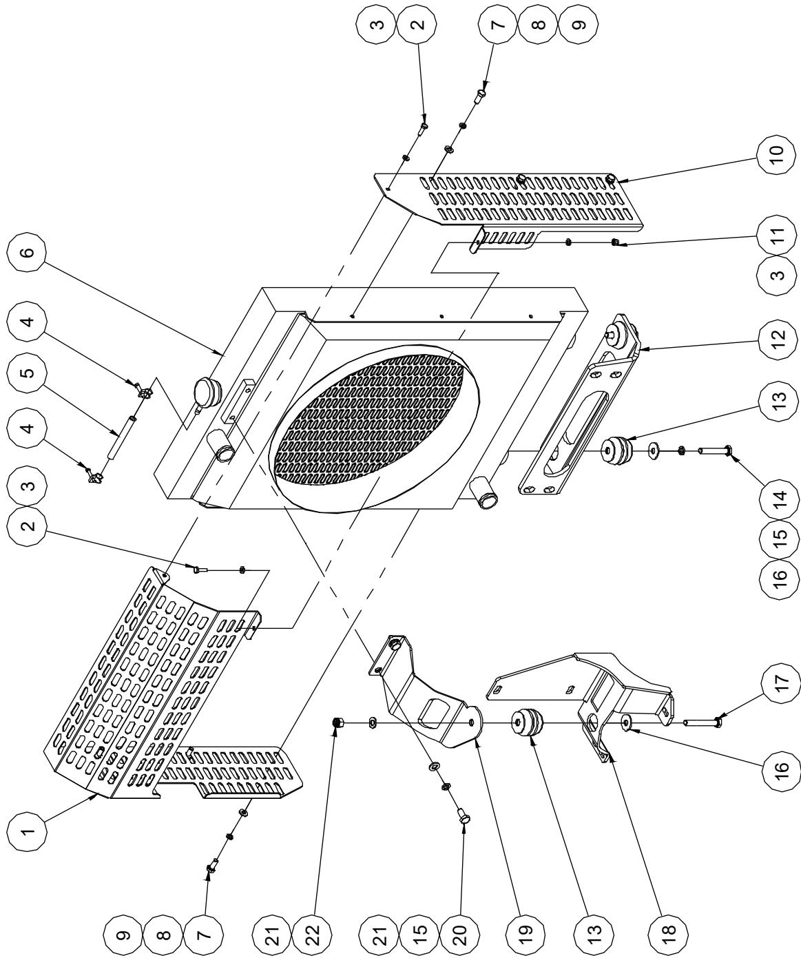
**112.1 Cooling System Assembly (Kubota EU Stage V Engine)**
