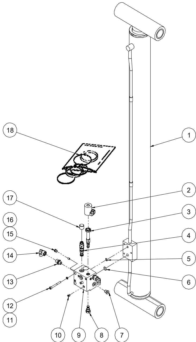
**402.1 Upper Lift Cylinder Assembly (JCPT1823RTB)**
