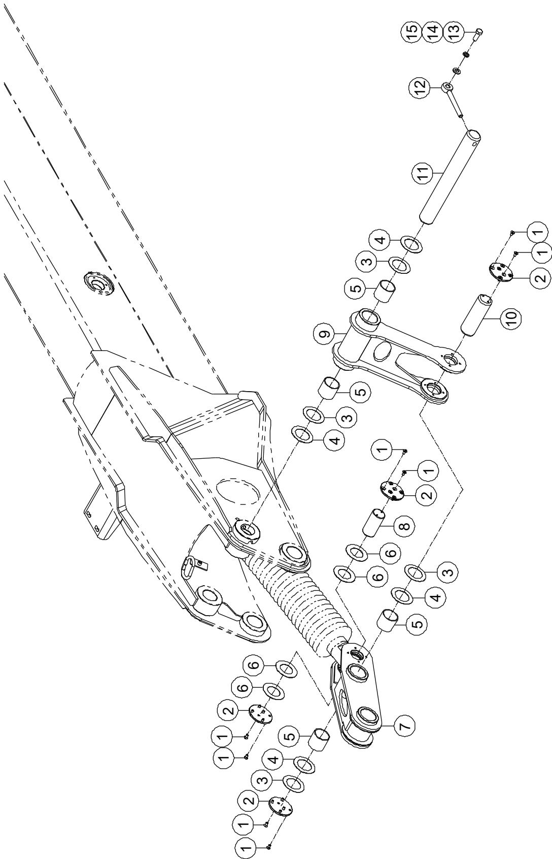
**3-20 Telescopic Boom and Linkage Installations (BT34BRT)**
