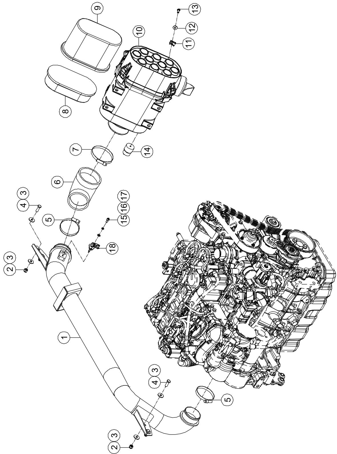
**1-23 Engine Suction System Installations (Stage V)**
