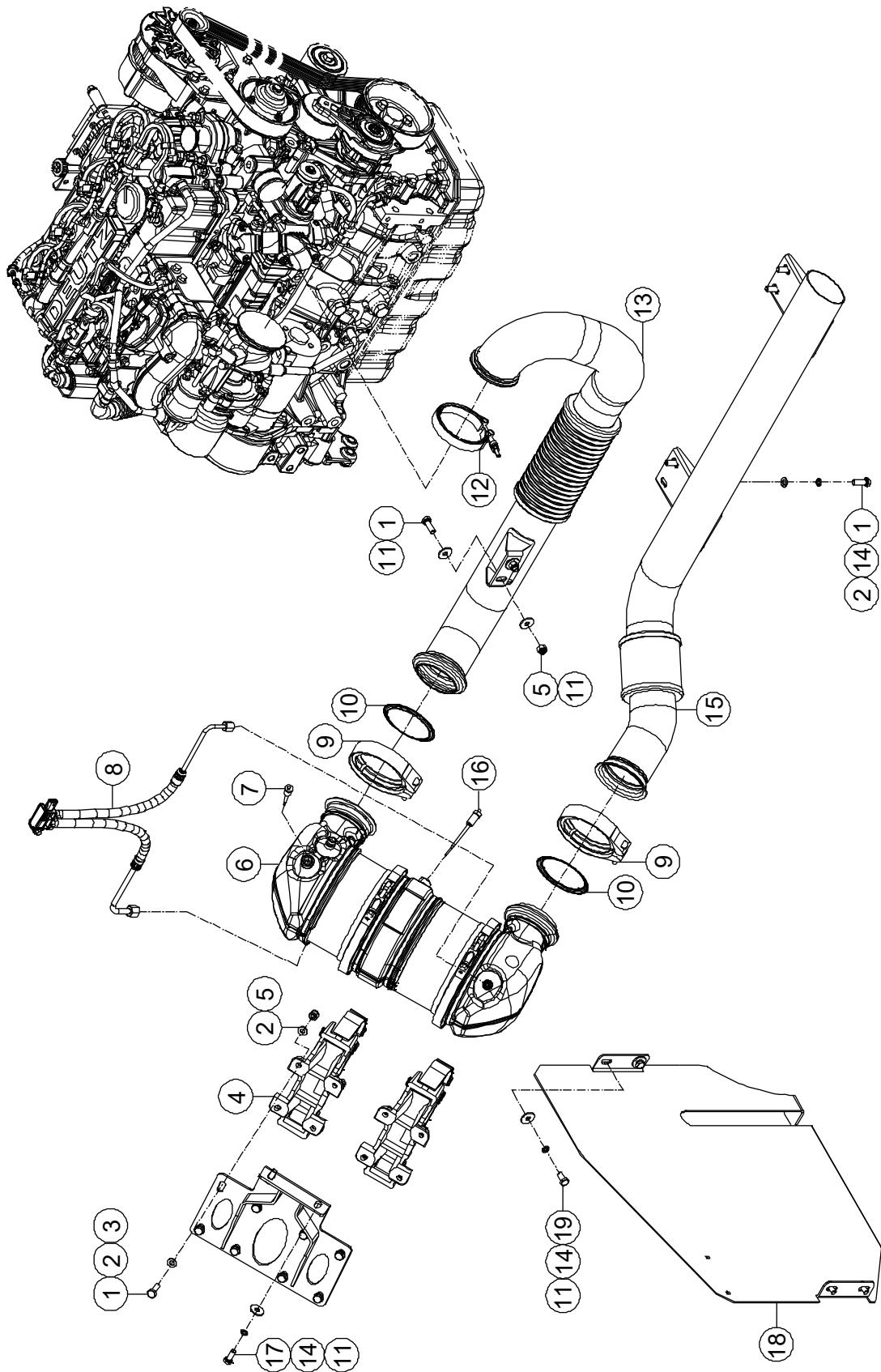
**1-24 Engine Exhaust System Installations (Stage V )**
