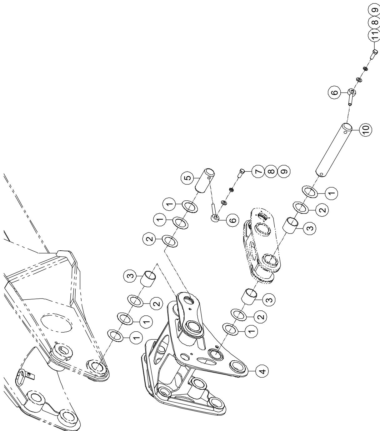
**3-21 Telescopic Boom and Articulating JIB Installations (BT34BRT)**
