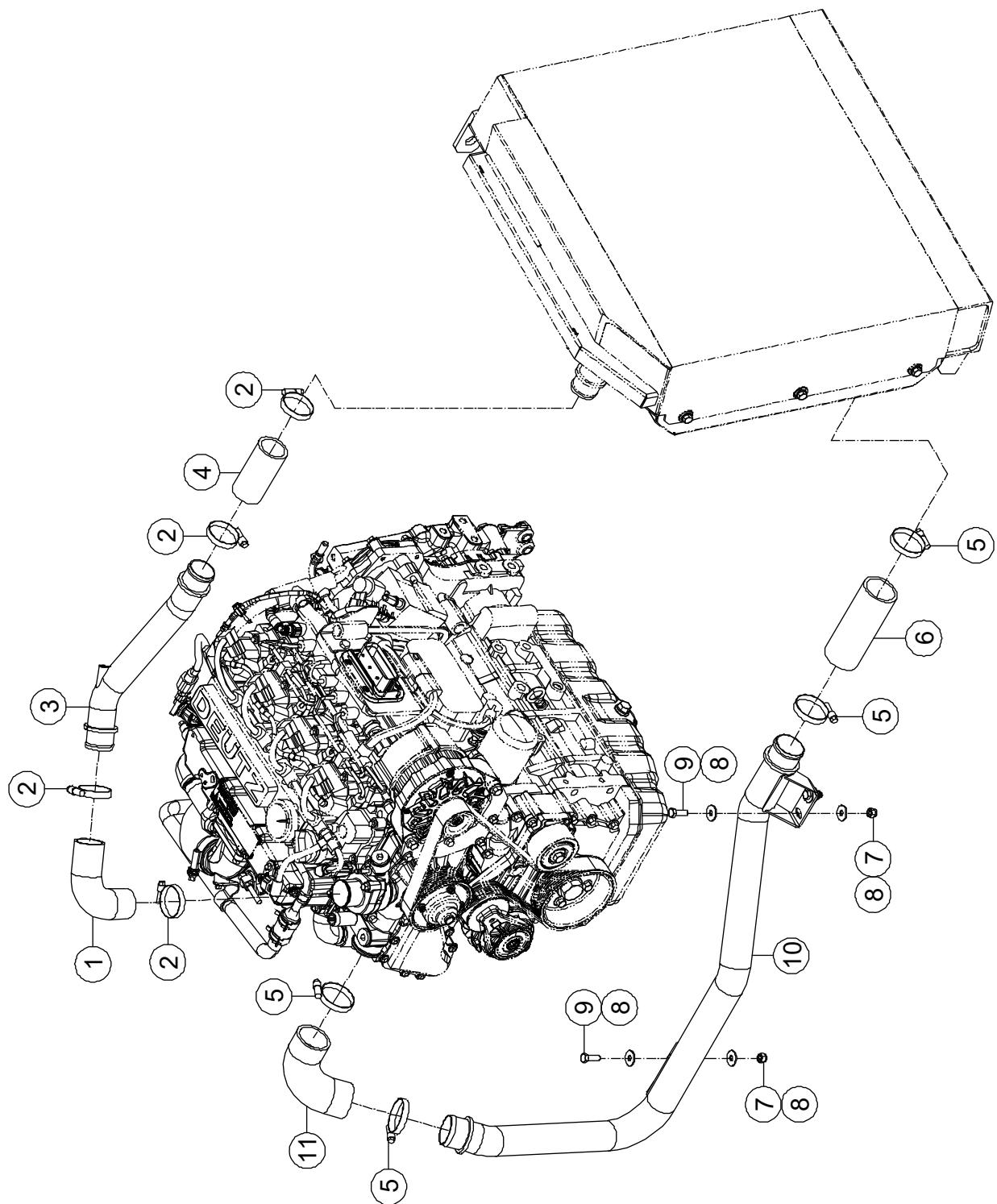
**1-17 Engine Cooling System Installations 3**
