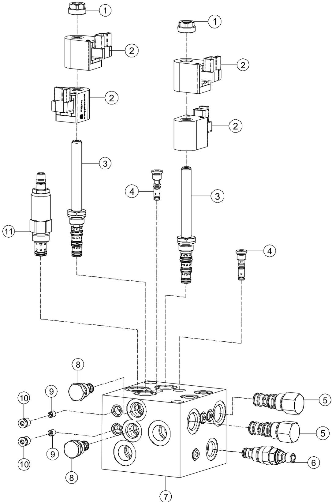
**3-32 Valve Block (BT30RT, BT28RT, BT26RT, BT24RT, BT28BRT, BT26BRT, BT24BRT)**
