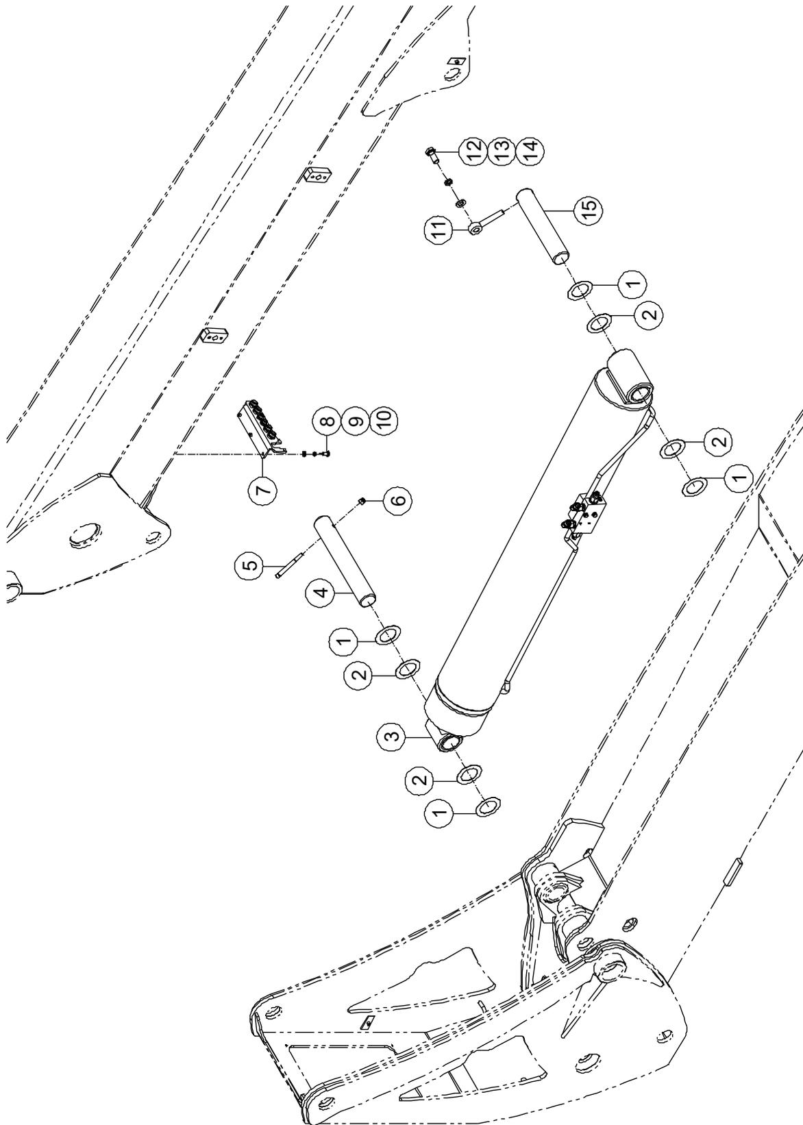
**3-4 Lifting Cylinder Assembly and Boom Installations**
