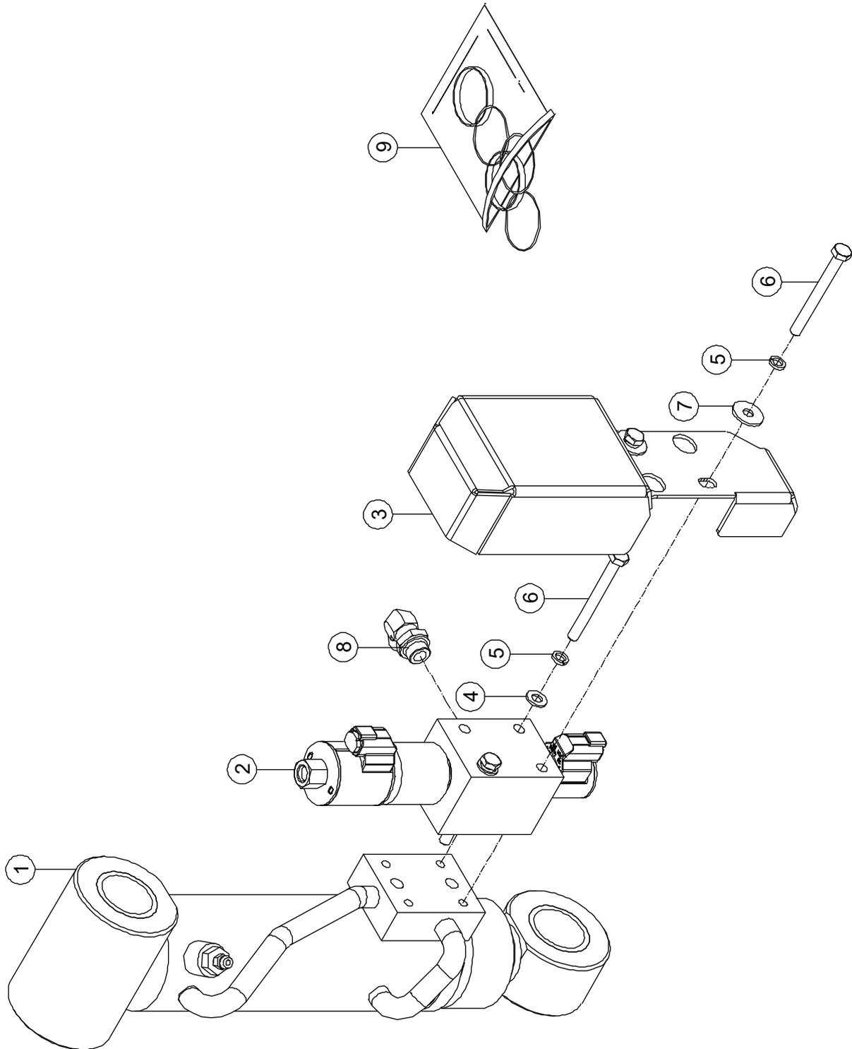
**5-1 Left Axle Lockout Cylinder Assembly**
