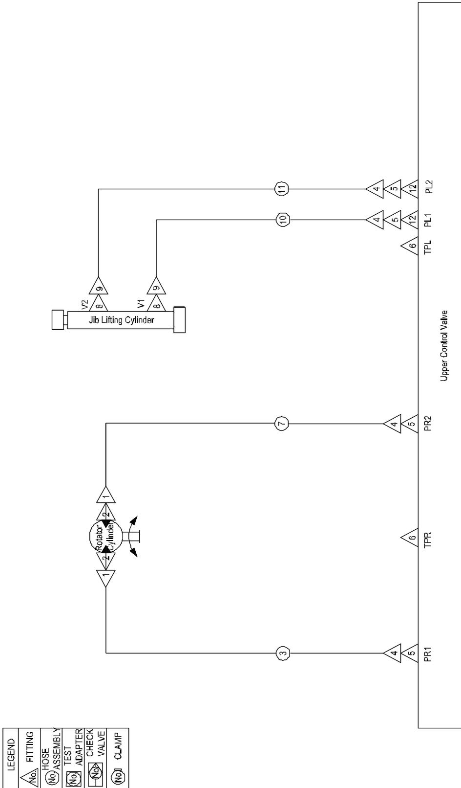
**6-5 JIB Circuit (BT30RT, BT28RT, BT26RT, BT24RT, BT28BRT, BT26BRT, BT24BRT)**
