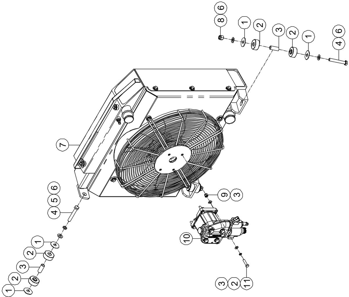
**1-13 Engine Cooling System Installations 1**
