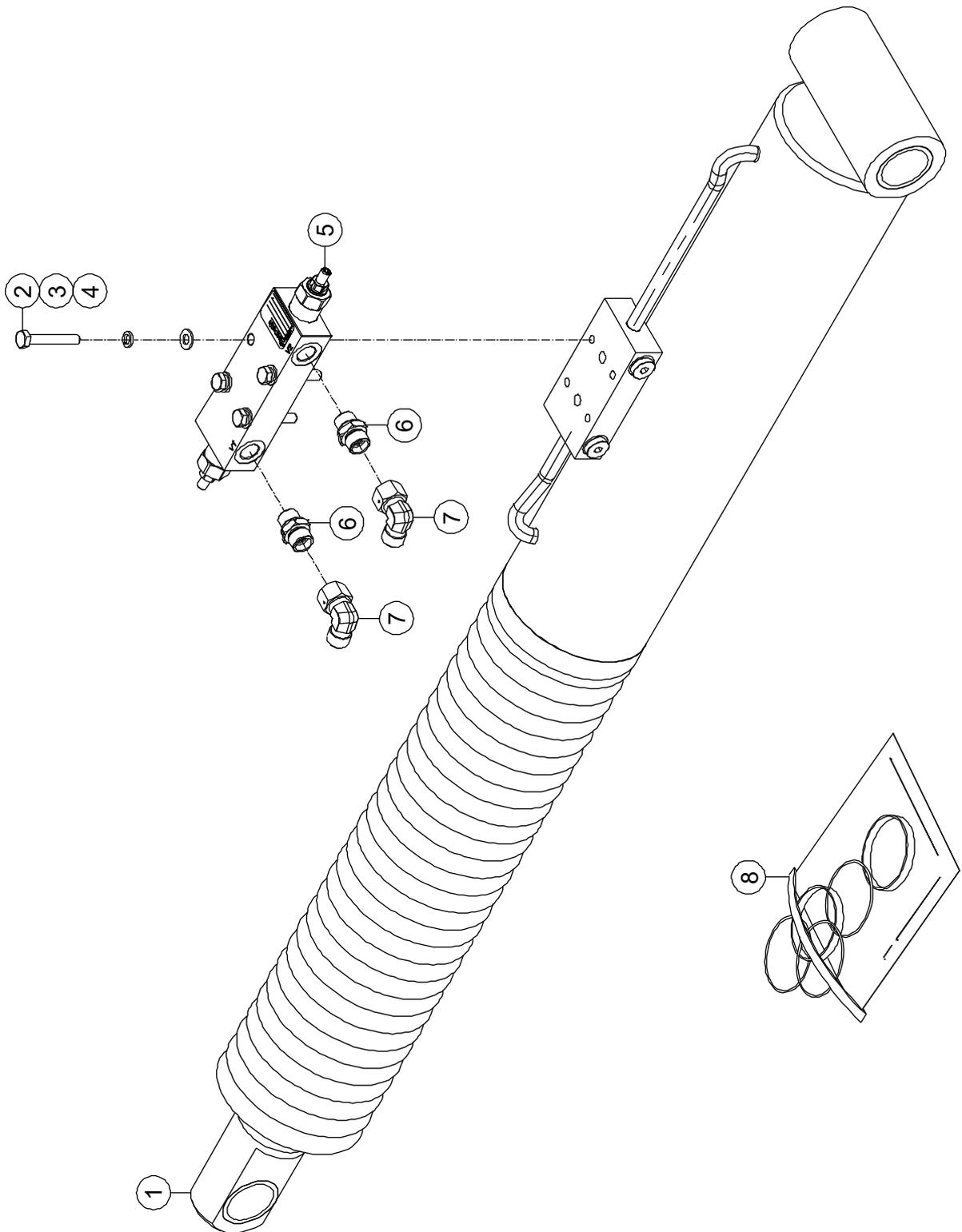
**5-6 JIB Leveling Cylinder Assembly (BT28BRT, BT26BRT, BT24BRT)**
