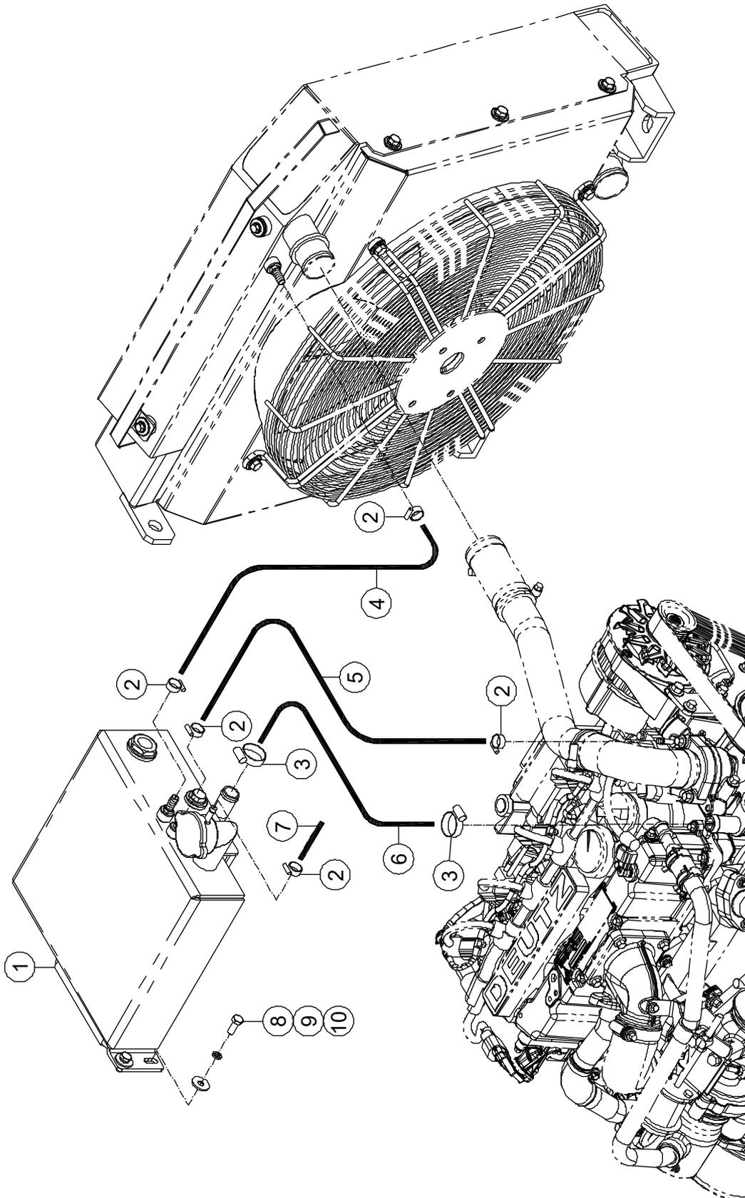
**1-15 Engine Cooling System Installations 2 (Stage IV)**
