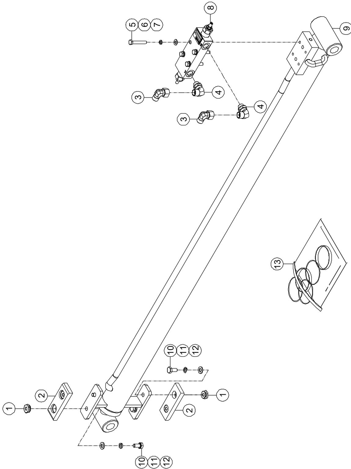
**5-8 JIB Telescopic Cylinder Assembly (BT30SRT, BT28SRT, BT26SRT)**
