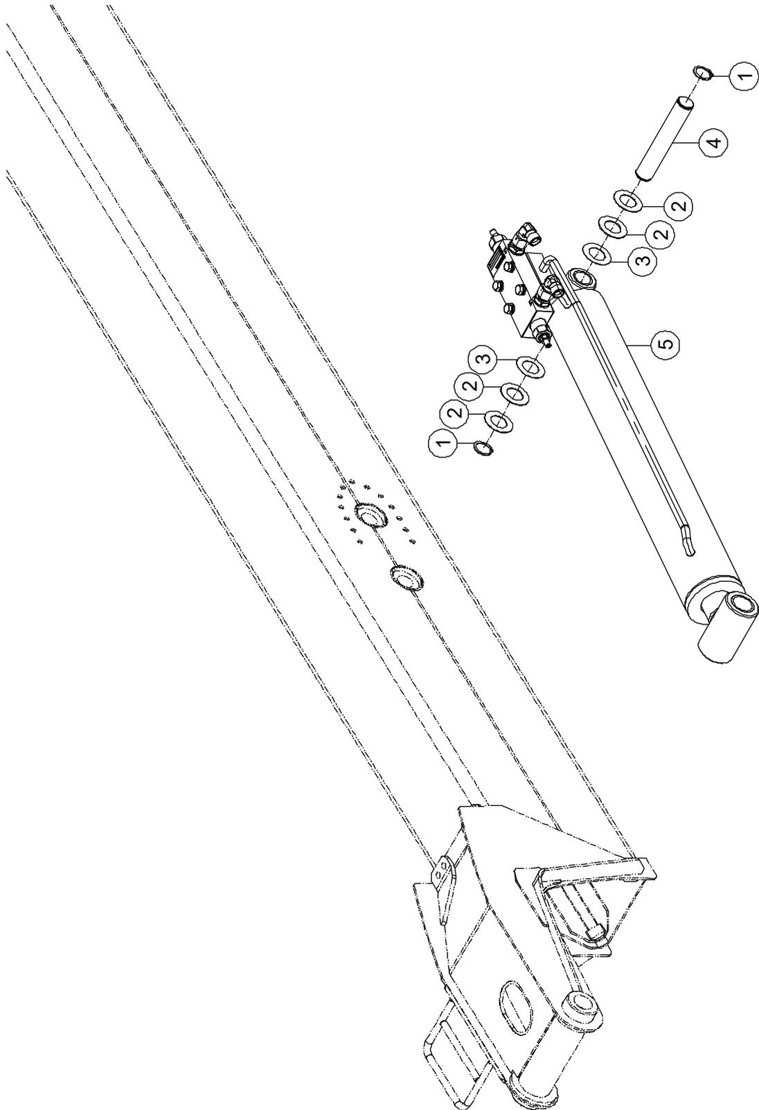
**3-23 Slave Cylinder Assembly Installations (BT30SERT, BT28SERT, BT26SERT)**
