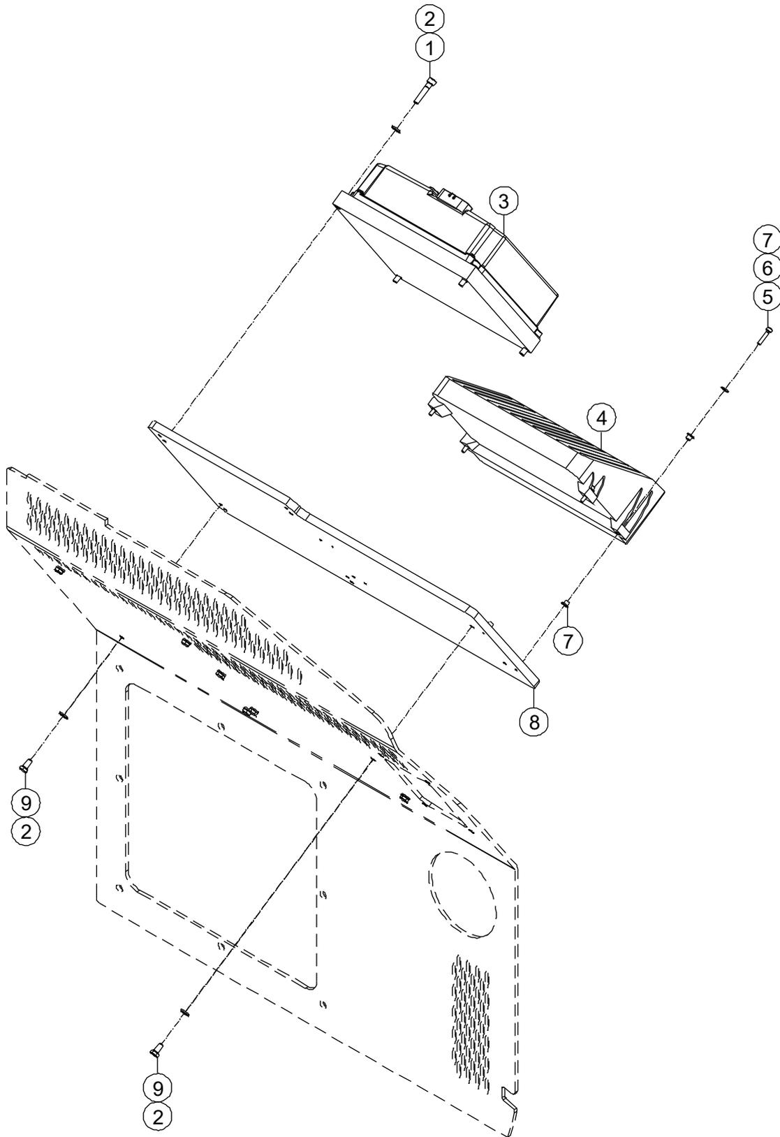
**7-3 Controller Assembly - COBO Controller**
