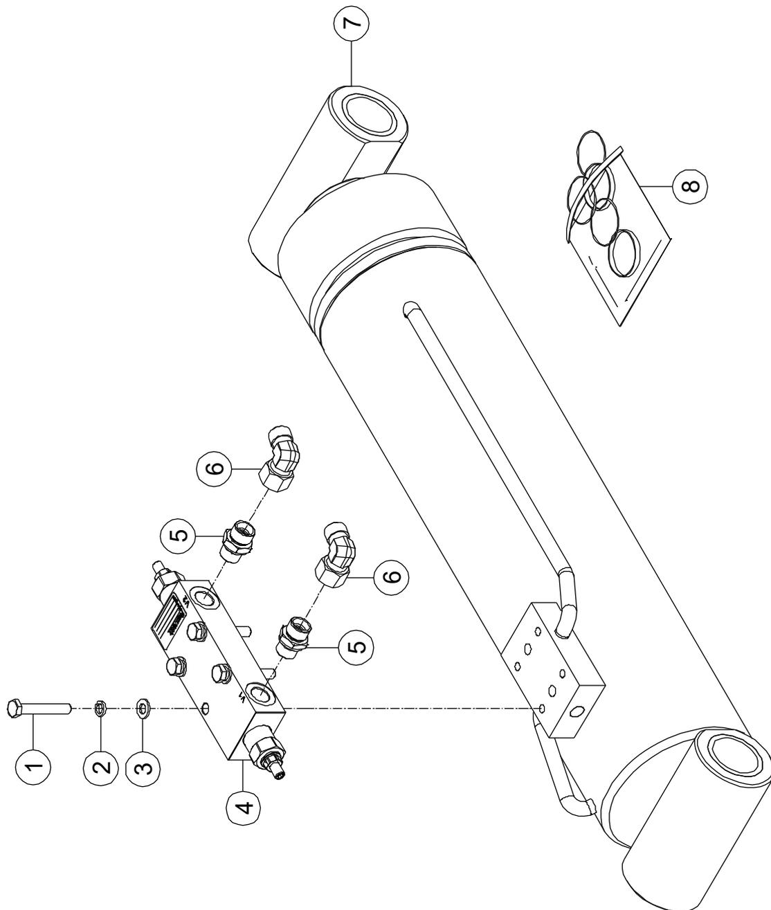
**5-7 JIB Leveling Cylinder Assembly (BA28RT, BA24RT)**
