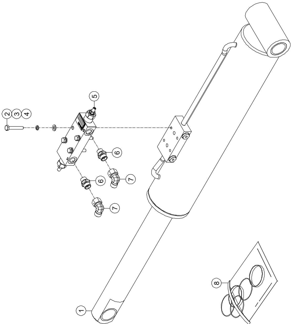
**5-8 JIB Leveling Cylinder Assembly (BA28BRT, BA24BRT)**
