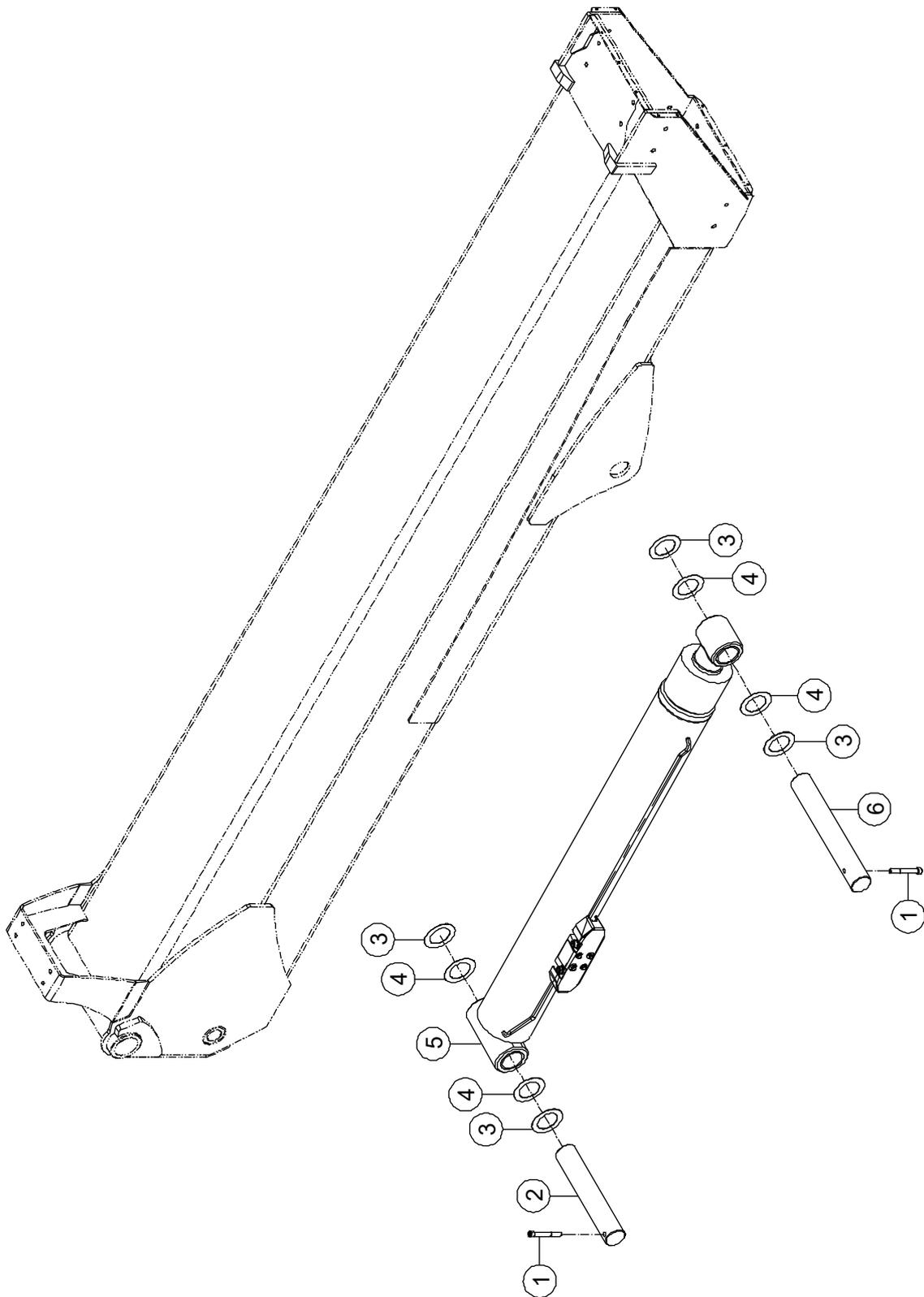
**3-3 Tower Lifting Cylinder Assembly Installations**
