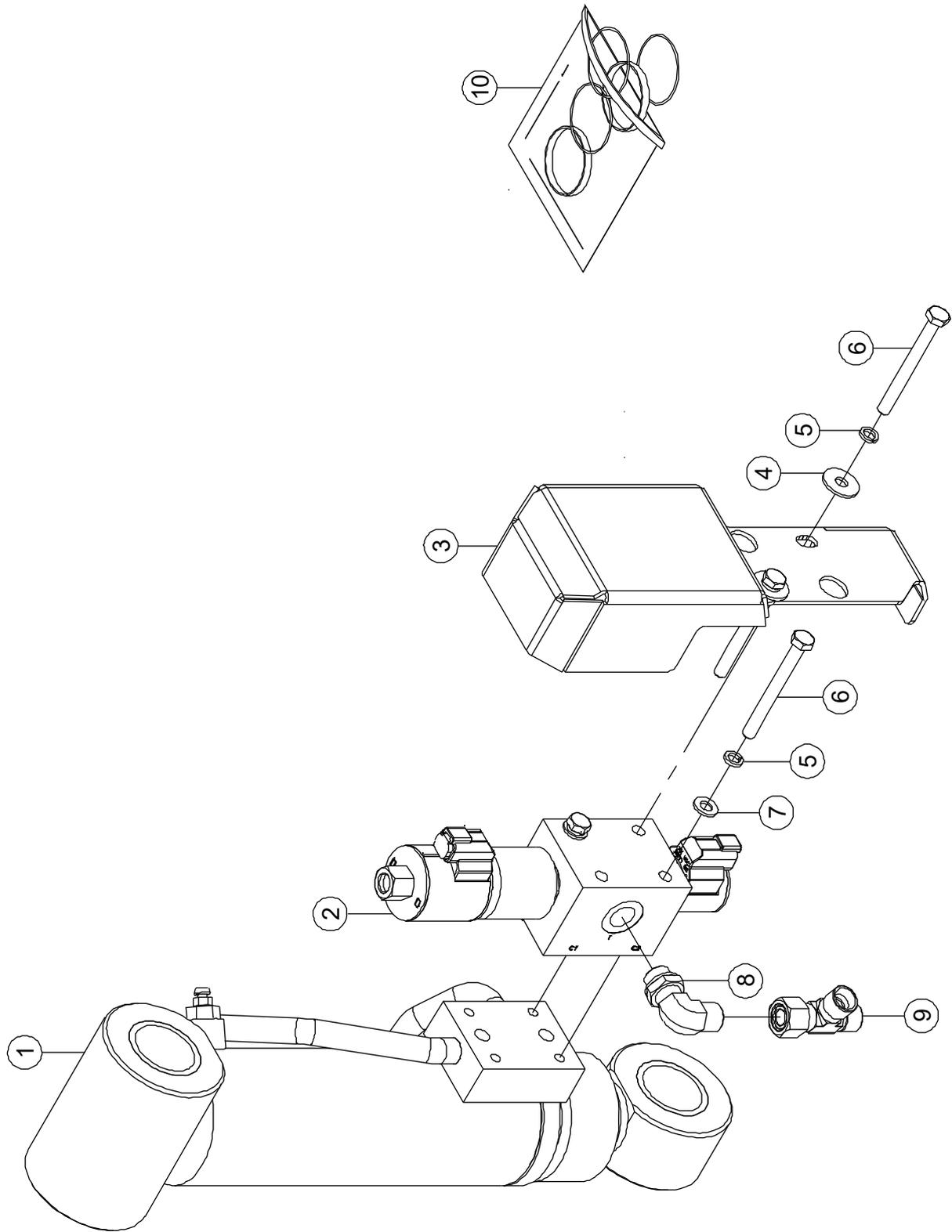
**5-2 Right Axle Lockout Cylinder Assembly**
