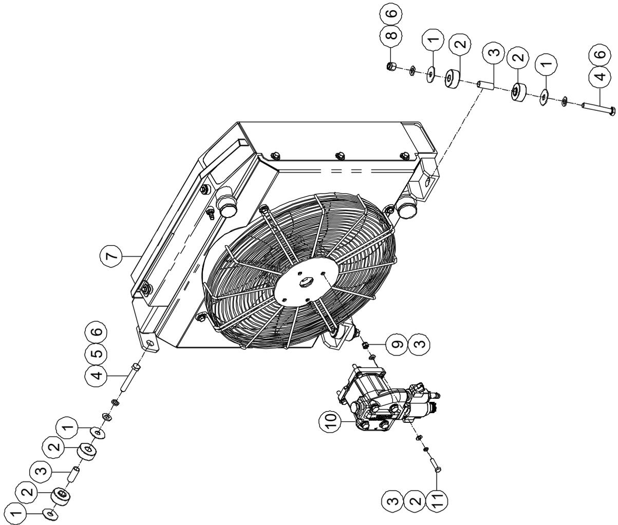
**1-13 Engine Cooling System Installations 1**
