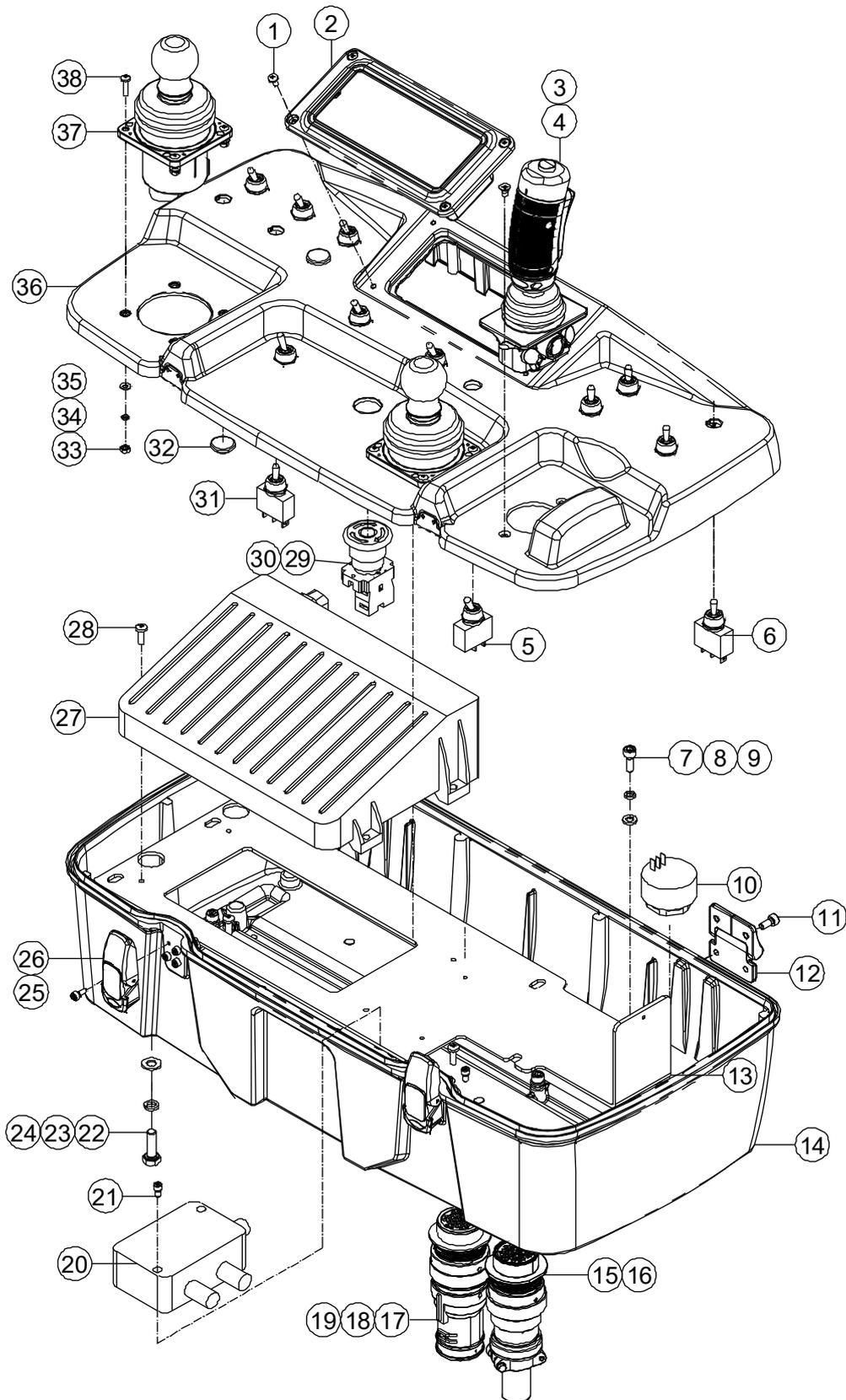
**7-8 Ground Control Panel Assembly - COBO Controller**
