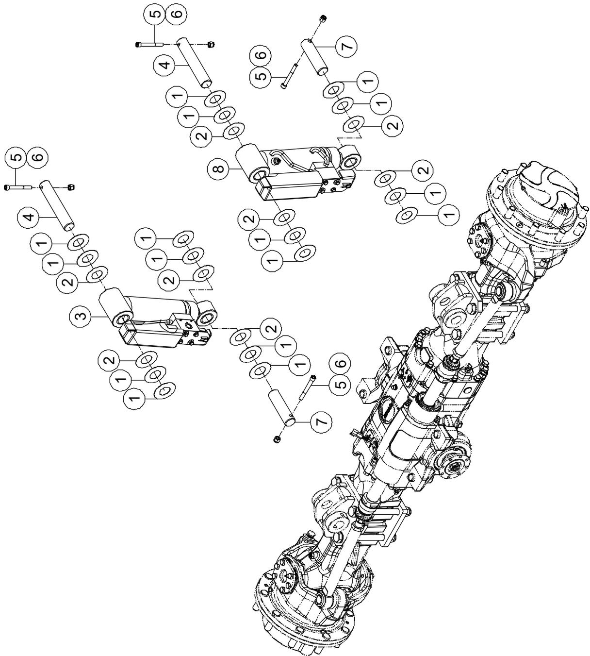
**1-2 Axle Lockout Cylinder Installations**
