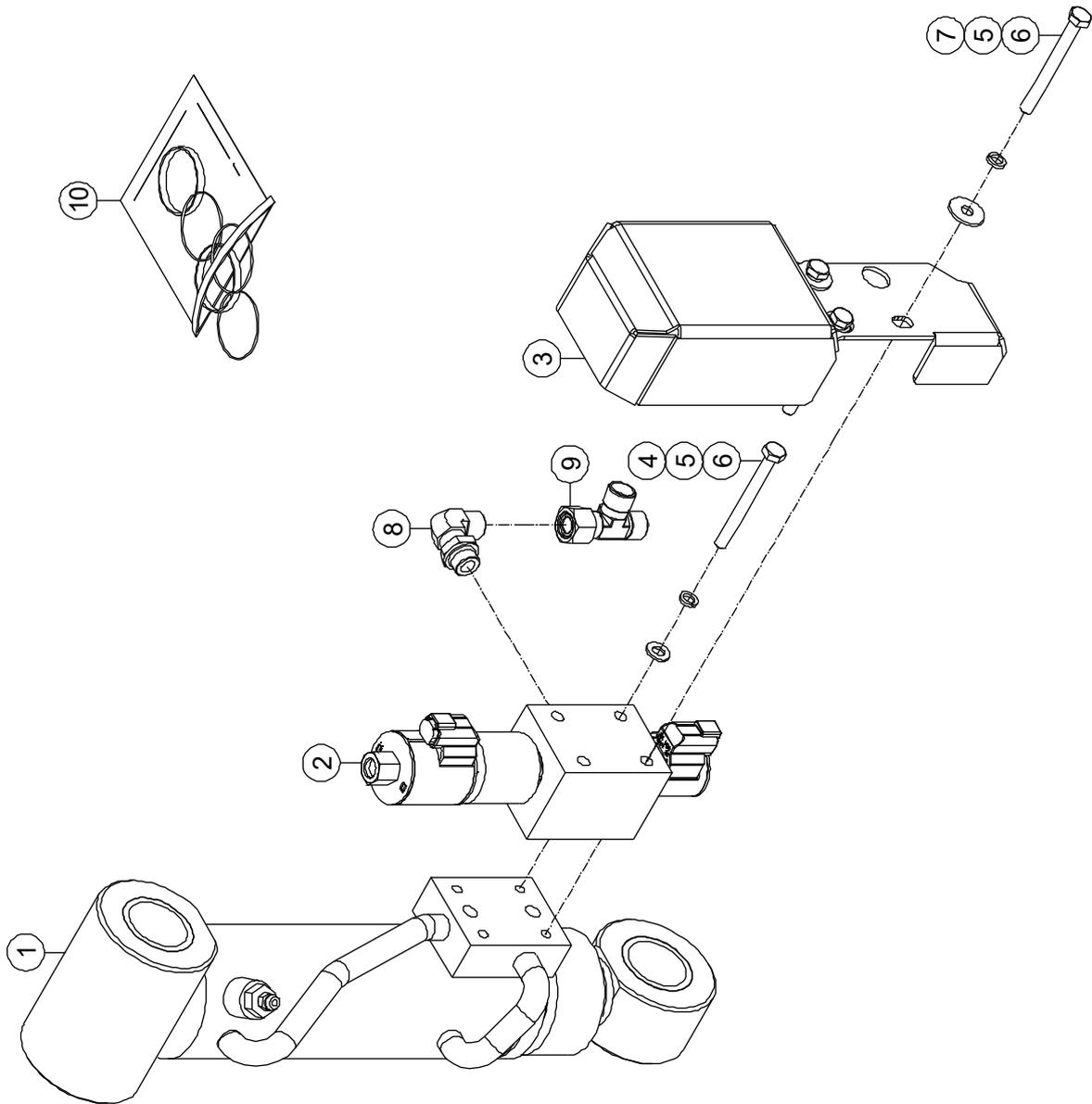
**5-1 Left Axle Lockout Cylinder Assembly**
