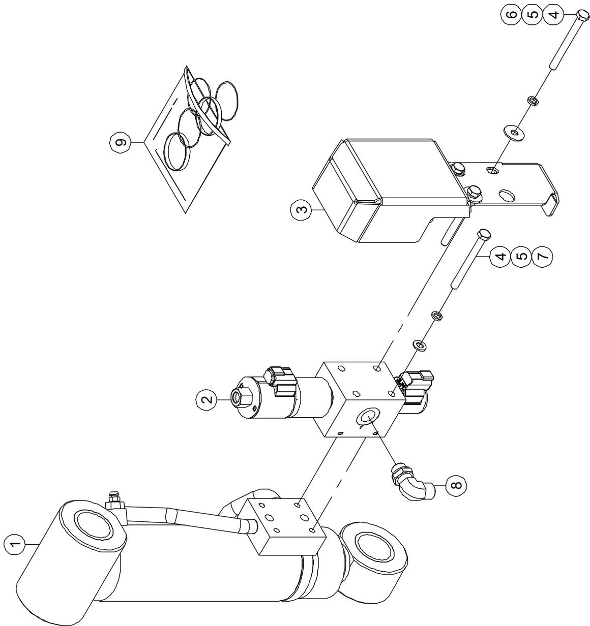
**5-2 Right Axle Lockout Cylinder Assembly**
