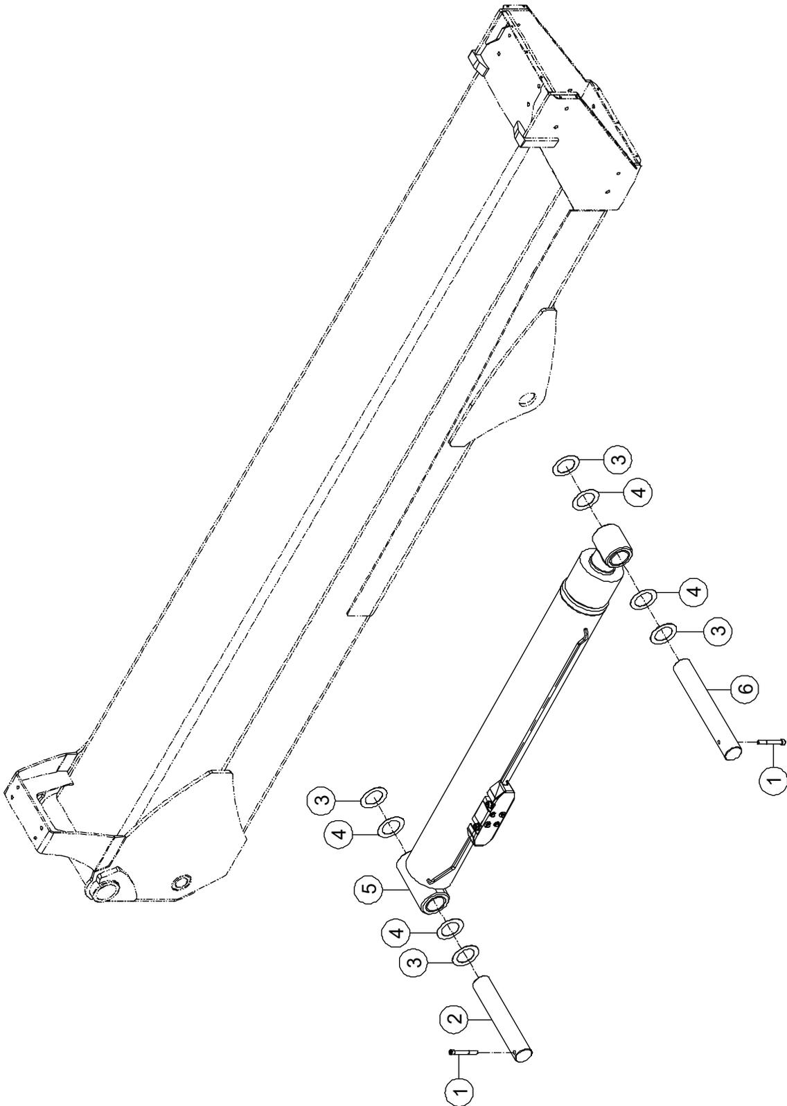
**3-3 Tower Lifting Cylinder Assembly Installations**
