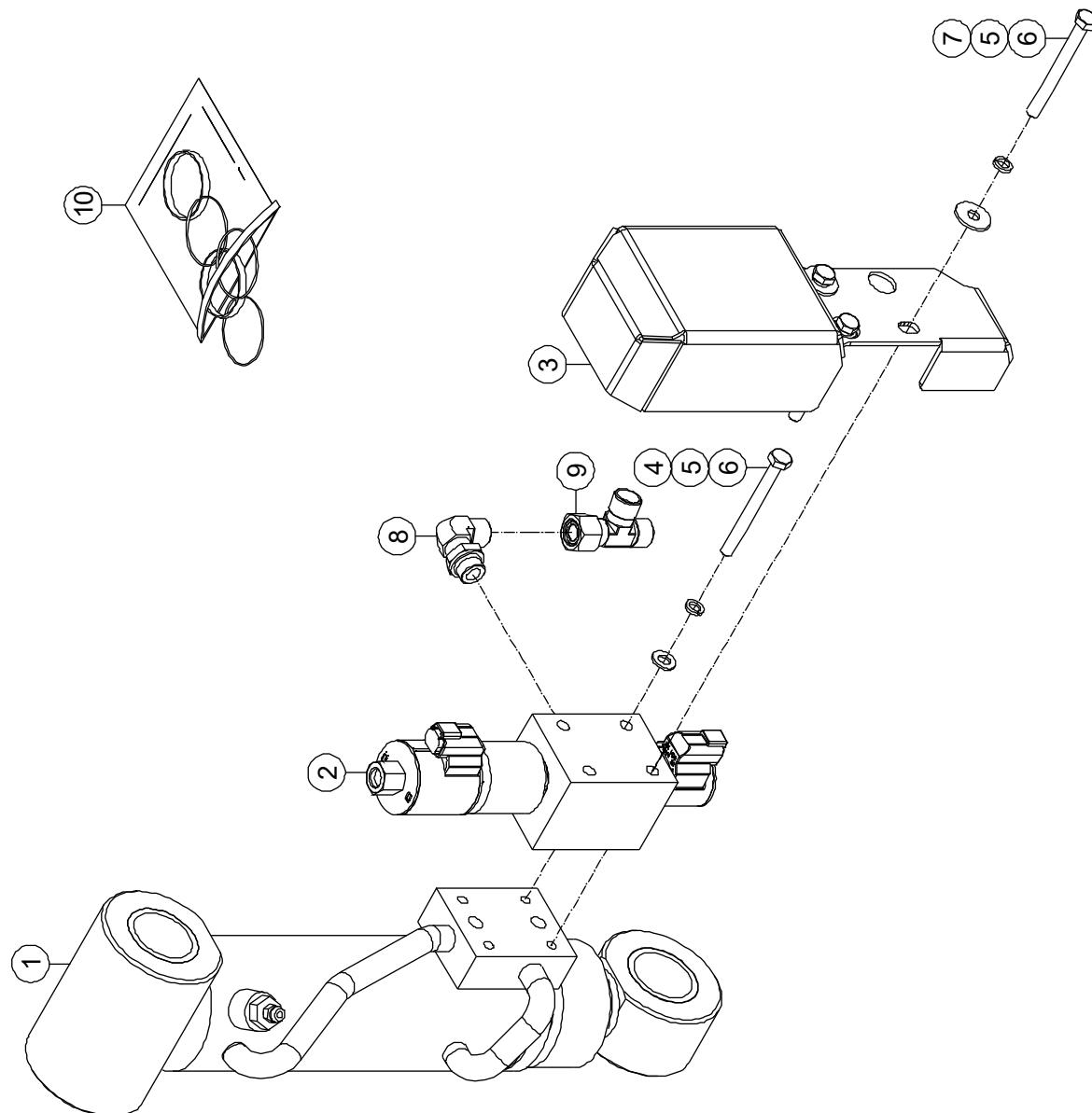
**5-1 Left Axle Lockout Cylinder Assembly**
